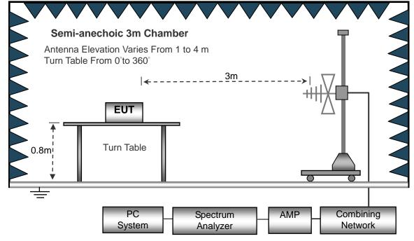
(C) Radiated Emission Test-Up Frequency Above 1GHz
