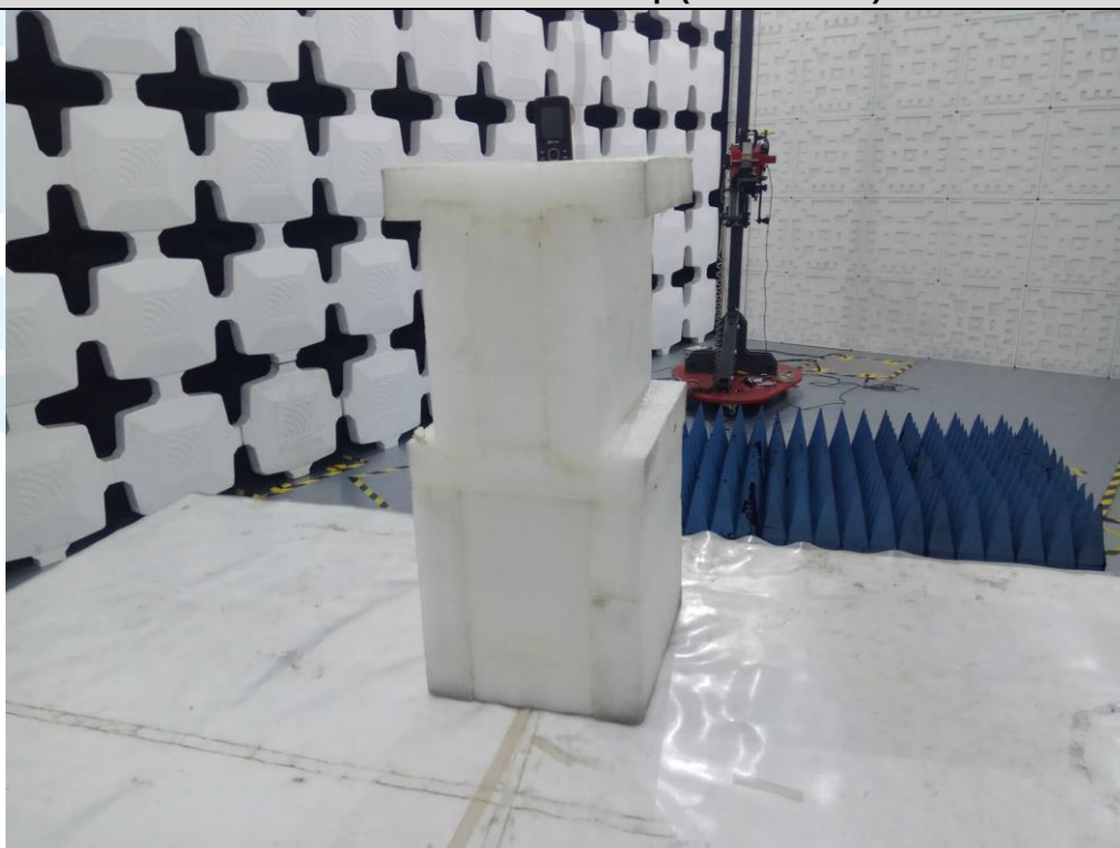
Radiated emission Test Setup (Above 1 GHz)
