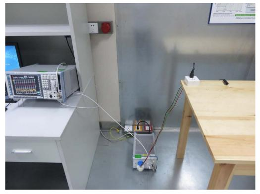
FCC RADIATED EMISSION TEST SETUP
