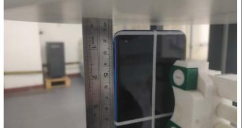
Back Side With Earphone (Separation distance of 10mm)
