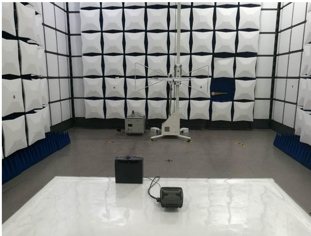
FCC RADIATED EMISSION TEST SETUP
