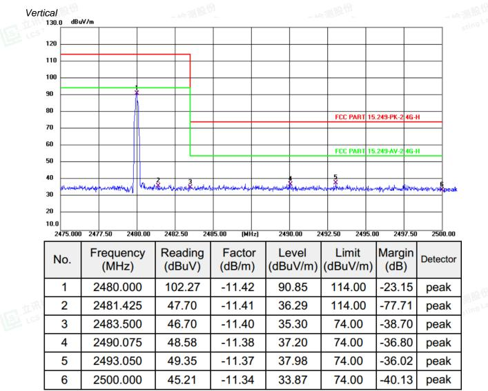
Note: Due to the measure PK emission level less than the AV limit value. No necessary to take down the AV emission level.
