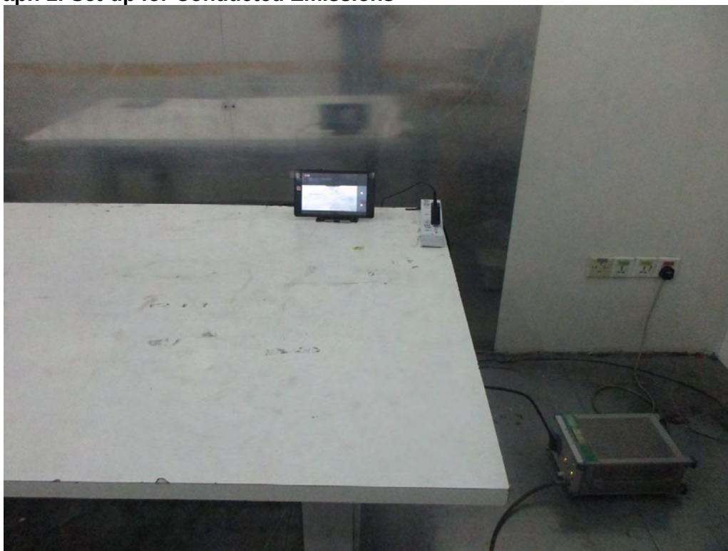
Photograph 2: Set-up for Spurious Emissions for below 30MHz
