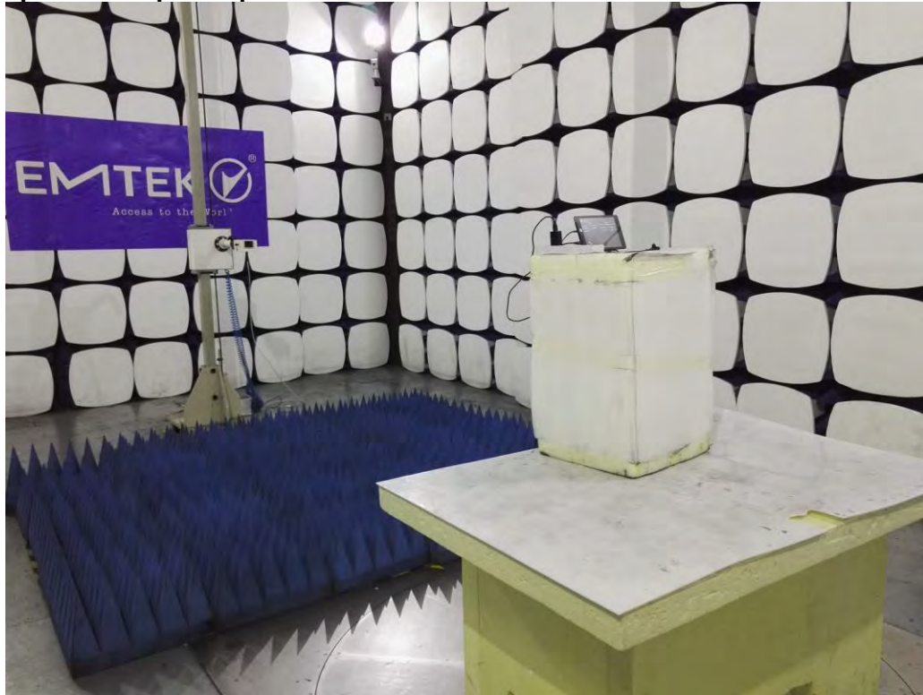
Photograph 5: Set-up for Spurious Emissions for 18 - 26.5GHz
