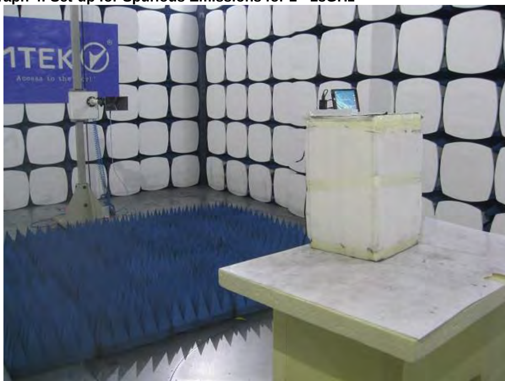
Photograph 4: Set-up for Spurious Emissions for 1 - 18GHz
