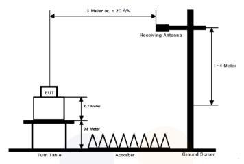
These measurements were performed at 3 m test site. The equipment under test is placed on a non-conductive table 1.5-meters above a turntable which is flush with the ground plance and 1.5 meters from the receive antenna. For measurements above 1 ( absorbers are placed on the floor between the turn table and the antenna mast in such a way so as to maximize the reduction of reflections. For measurements below 1 ( the absorbers are removed.
