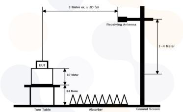
These measurements were performed at 3 test site. The equipment under test is placed on a nonconductive table 1.5-meters above a turntable which is flush with the ground plane and 3 meters(for below 1 GHz: 0.8-m) from the receive antenna. For measurements above 1 GHz absorbers are placed on the floor between the turn table and the antenna mast in such a way so as to maximize the reduction of reflections.
