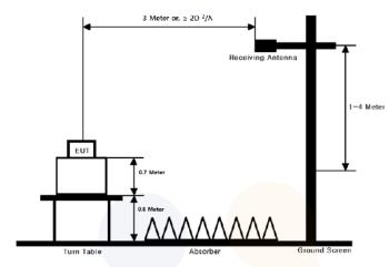
These measurements were performed at 3 m test site. The equipment under test is placed on a non-conductive table 1.5-meters above a turntable which is flush with the ground plance and 1.5 meters from the receive antenna. For measurements above 1 GHz absorbers are placed on the floor between the turn table and the antenna mast in such a way so as to maximize the reduction of reflections. For measurements below 1 GHz, the absorbers are removed.
