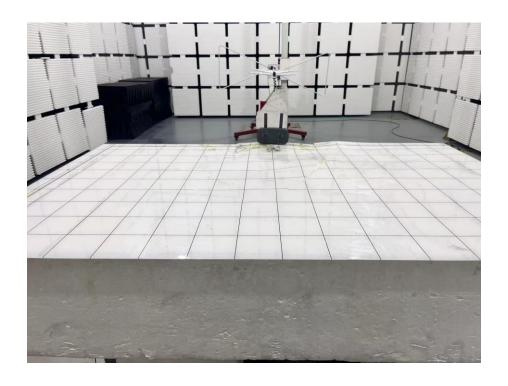
Set-up for Radiated Spurious Emission, Above 1GHz
