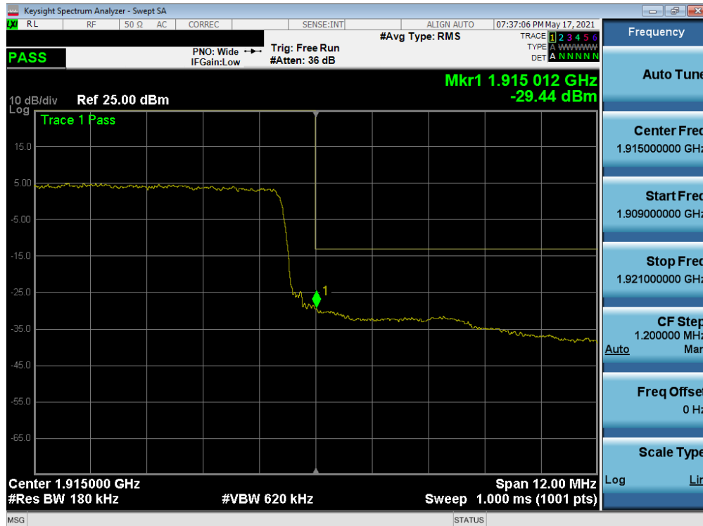
Plot 7-53. Upper Band Edge Plot (LTE Band 25 - 15MHz QPSK – Full RB)
