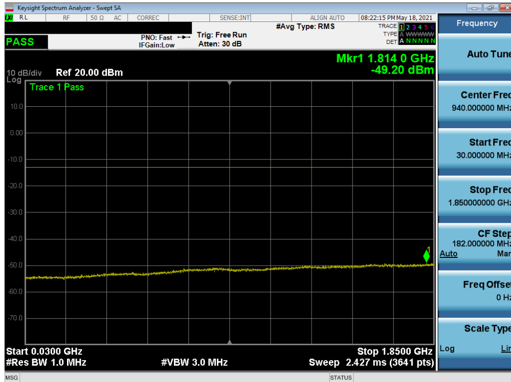
Plot 7-40. Conducted Spurious Plot (WCDMA Ch. 9538)
