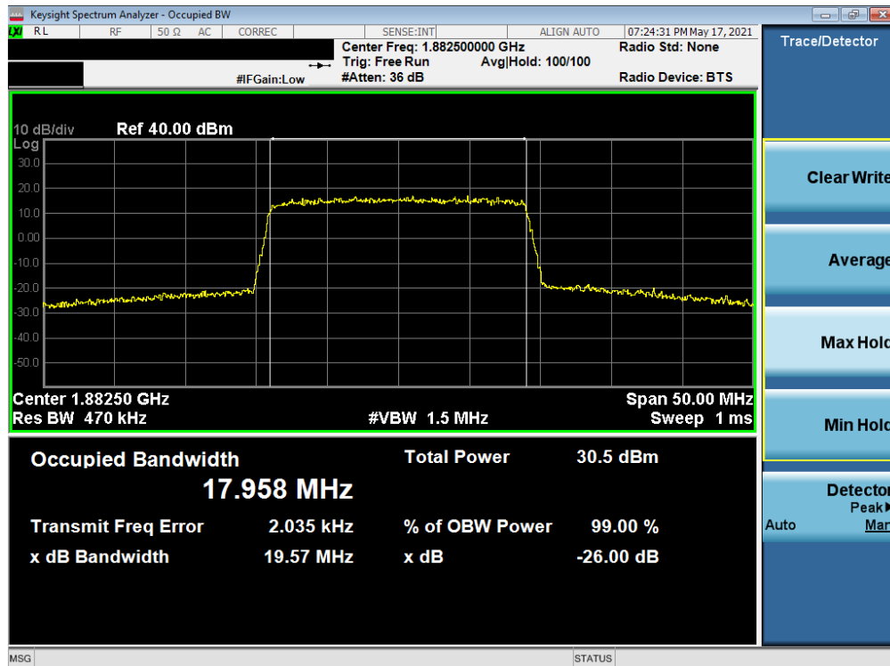
Plot 7-2. Occupied Bandwidth Plot (LTE Band 25/2 - 20MHz 16-QAM - Full RB)
