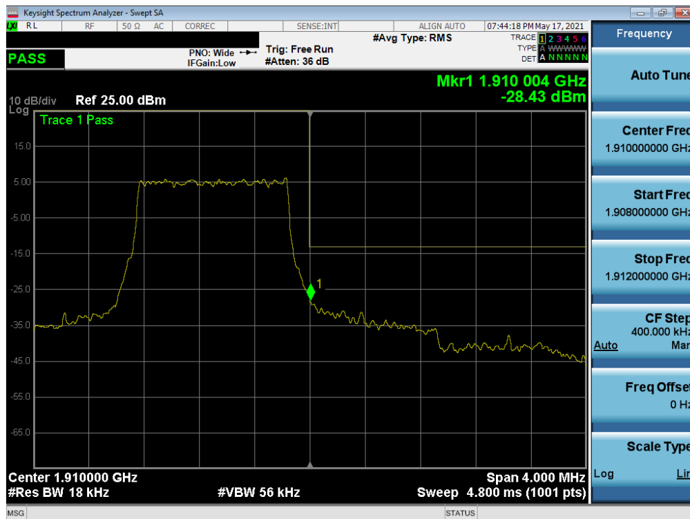
Plot 7-75. Upper Band Edge Plot (LTE Band 2 – 1.4MHz QPSK – Full RB)
