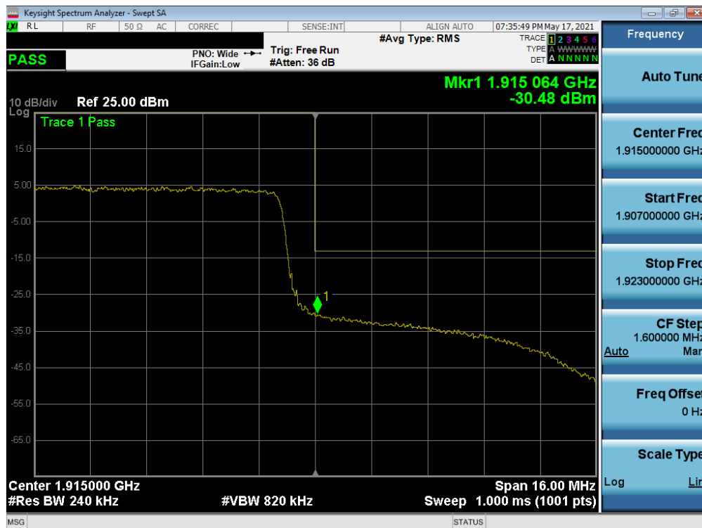
Plot 7-47. Upper Band Edge Plot (LTE Band 25 - 20MHz QPSK – Full RB)
