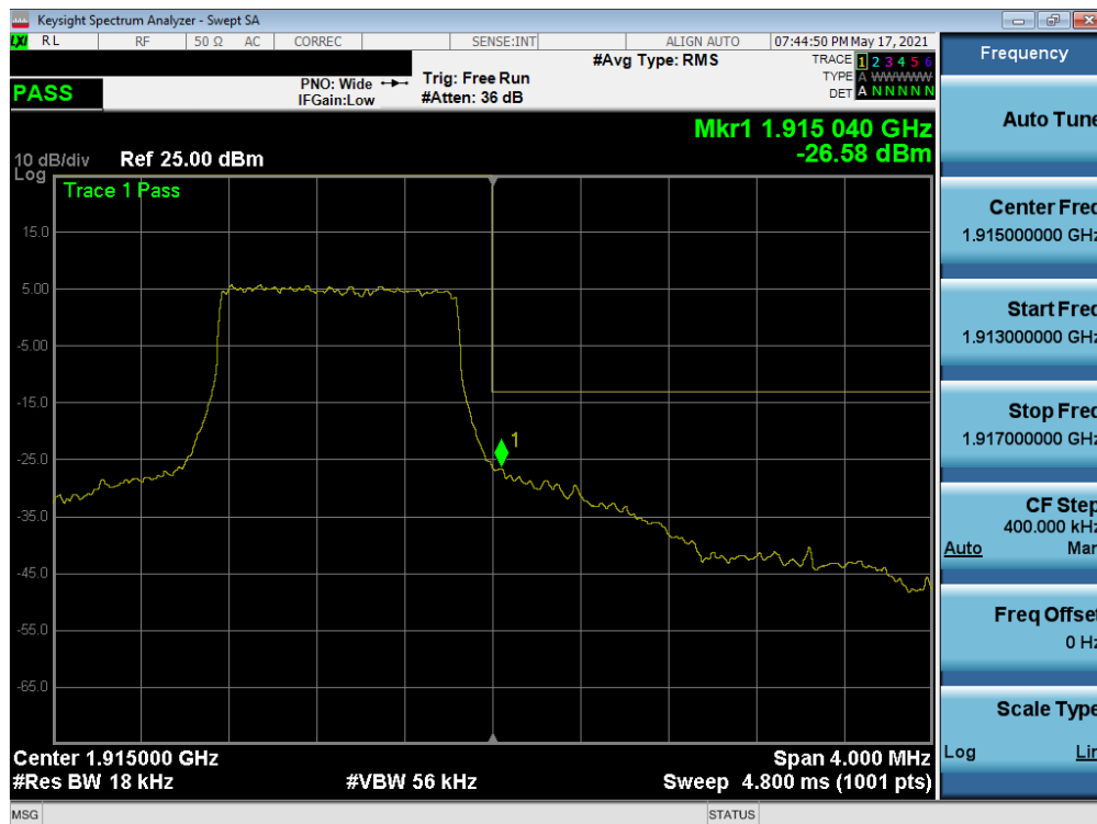
Plot 7-77. Upper Band Edge Plot (LTE Band 25 – 1.4MHz QPSK – Full RB)
