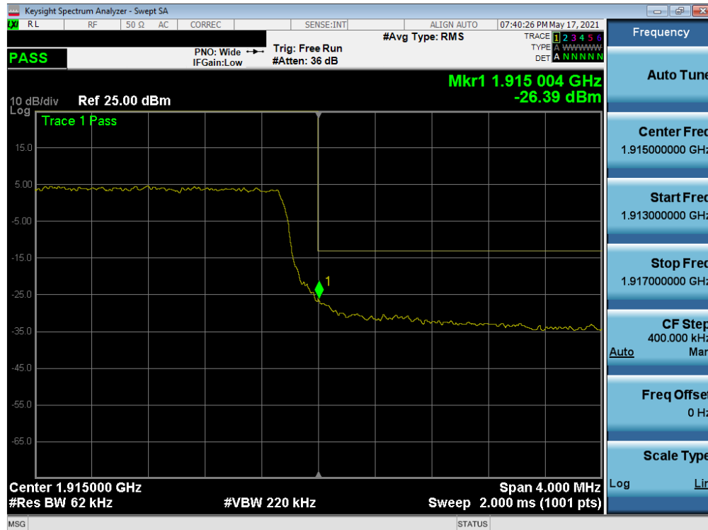
Plot 7-65. Upper Band Edge Plot (LTE Band 25 - 5MHz QPSK – Full RB)
