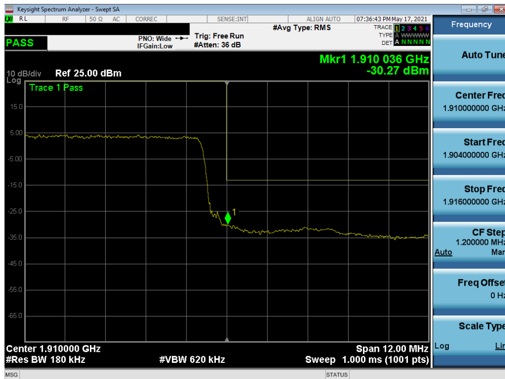
Plot 7-51. Upper Band Edge Plot (LTE Band 2 - 15MHz QPSK – Full RB)
