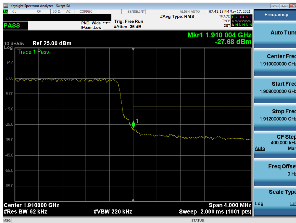
Plot 7-63. Upper Band Edge Plot (LTE Band 2 - 5MHz QPSK – Full RB)
