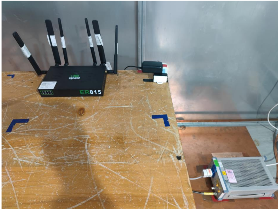
Conducted Emissions Test Setup (with charger)
