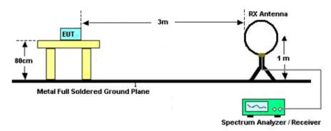
For radiated emissions from 30MHz to 1GHz
