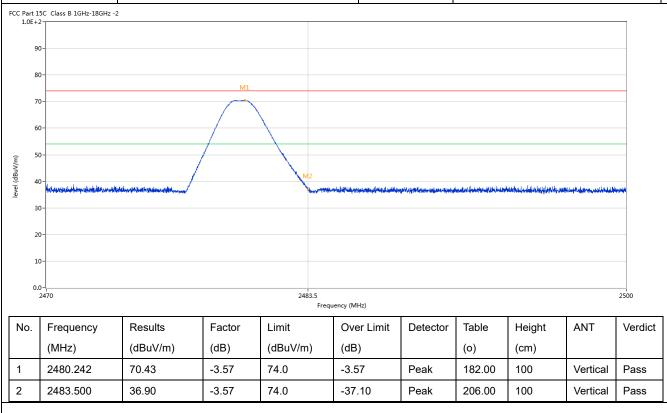
Note: 1. The PK emission level less than the AV limit. No necessary to record the AV emission level.
