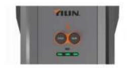
3.3.2 Then press the remote control button. When the hose reel receives a signal, the four LED lights will enter a long on state. Then press the 【STOP】 button to exit. If the four LED lights will turn off, it indicates that the remote control has been successfully paired.
