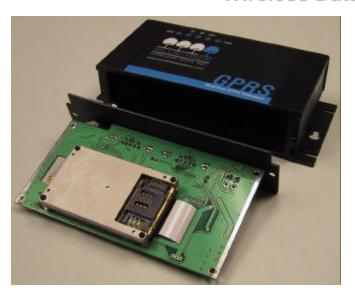
4- Open the SIM holder and insert the SIM card into it
