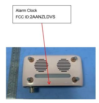
Note: The label is printed on the product by means of Spray paint.
