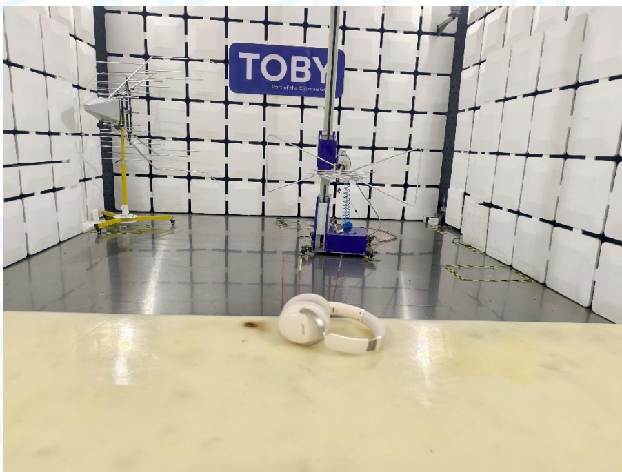
Photo of Setup for Radiated Emission (30MHz~1GHz)
