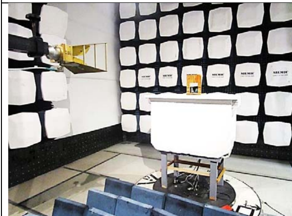
Radiated Emissions (>1GHz) – Front View
