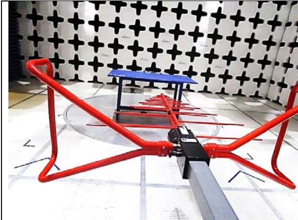
Radiated Emissions (<1GHz) – Front View
