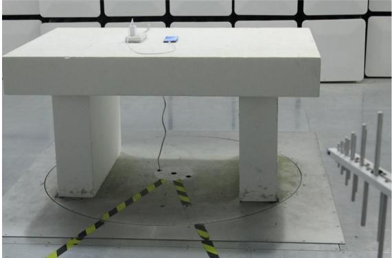
**1.4** Setup for Unwanted Emissions that fall Outside of the Restricted Bands(Radiated) and Unwanted Emissions in the Restricted Bands (Radiated) above 1GHz
