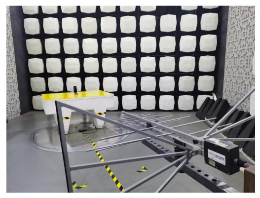
**1.2** Setup for Unwanted Emissions that fall Outside of the Restricted Bands(Radiated) and Unwanted Emissions in the Restricted Bands (Radiated) above 1GHz
