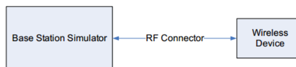
Figure 10.1 Power Measurement Setup
