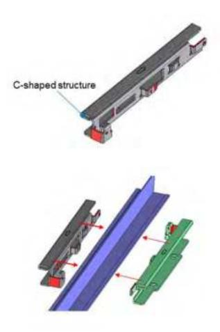
2. After the adapter brackets are affixed onto the T-bar, slide the brackets in the direction of the arrows on the brackets until they are securely attached to each other. Refer to the images below for how the adapter brackets should fit.
