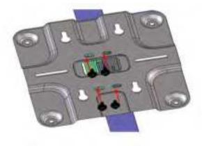
4. Align the screw holes on the main bracket with the corresponding holes on the back of the Access point, then use four M4 screws to attach the main bracket to the Access Point.
