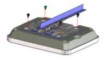
Note: Make sure the arrow on the main bracket is aligned so that it is pointing toward the top side of the Access Point.
