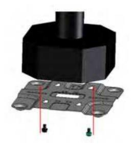
3. Align the screw holes on the main bracket with the corresponding holes on the back of the Access point, then use four M4 screws to attach the main bracket to the Access Point.
