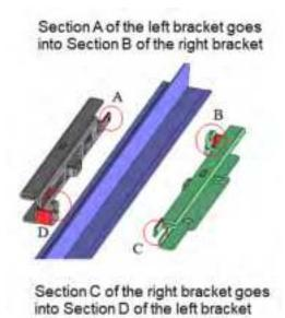
3. Align the screw holes on the adapter brackets with the holes on the main bracket (refer to section 2.2), then use four M3 screws to screw the main bracket to the adapter brackets.
