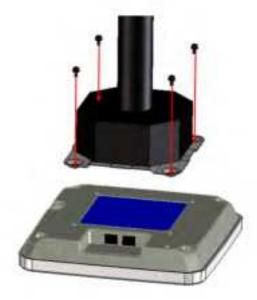
Note: Make sure the arrow on the main bracket is aligned so that it is pointing toward the top side of the Access Point.
