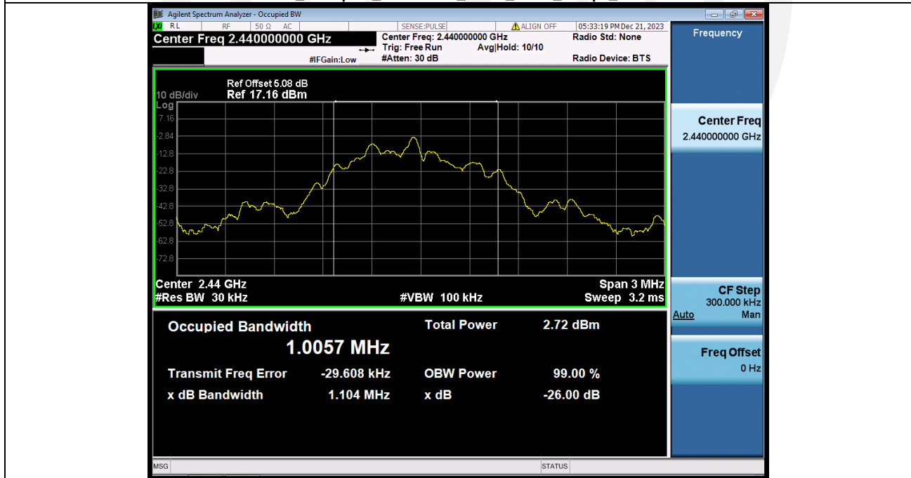
99% Occupied Bandwidth NVNT ANT1 1Mbps 2440
