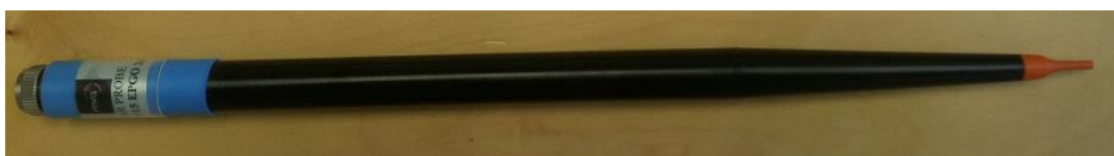
Figure 1 – MVG COMOSAR Dosimetric E field Dipole
