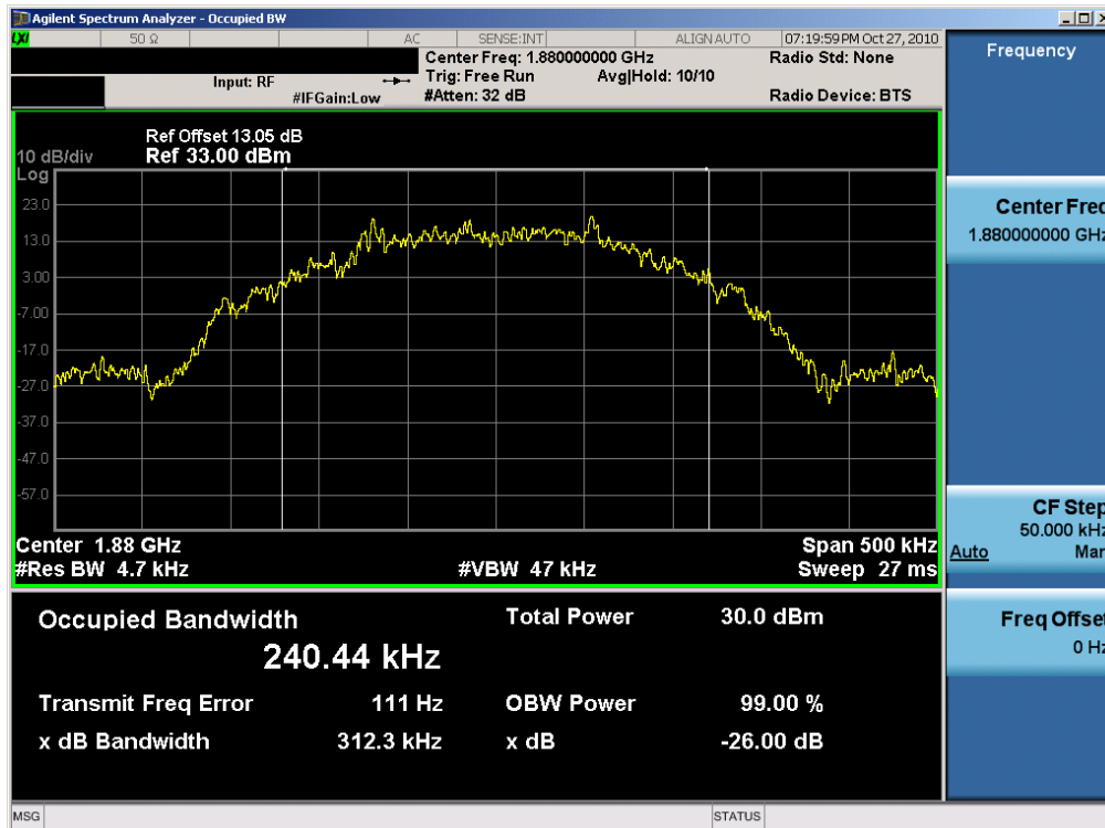
Plot 7-21. Occupied Bandwidth Plot (EDGE1900 Mode – Ch. 661)
