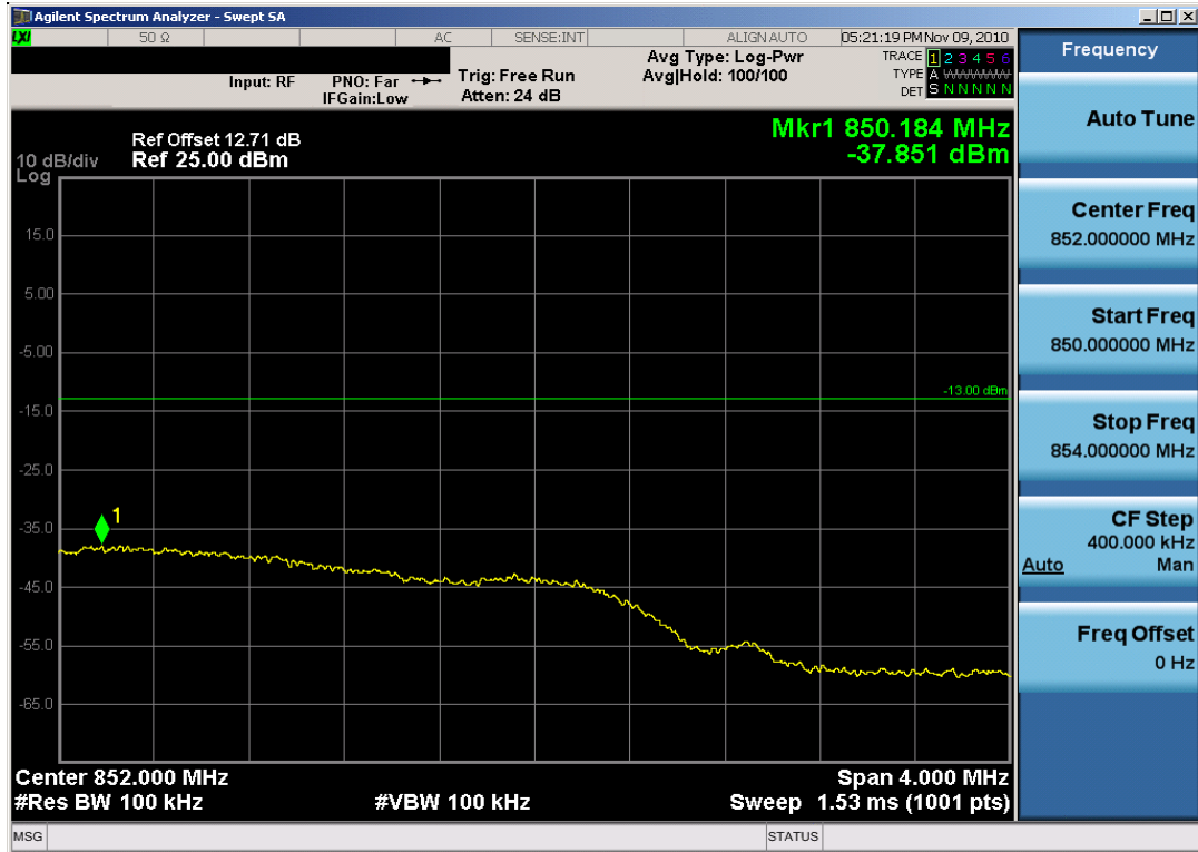
Plot 7-33. 4MHz Span Plot (Cellular WCDMA Mode – Ch. 4233)
