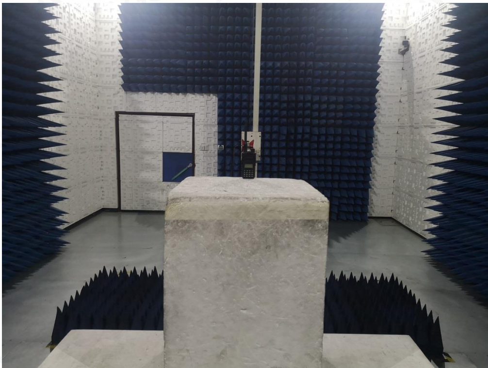
RADIATED EMISSION ABOVE 1G TEST SETUP
