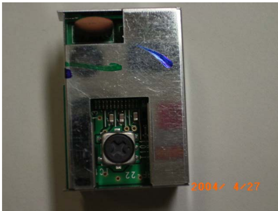
Tuner – Front with shield
