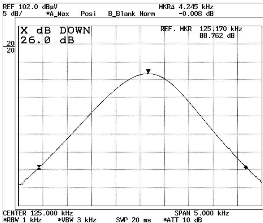
\* The measurement result data of 99% Occupied Bandwidth used the measurement result of -26dB Bandwidth.
