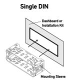
**Step 1:** Insert the mounting sleeve into the installation kit or dashboard.
