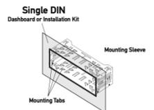
**Step 2:** Bend multiple mounting tabs around the mounting sleeve until the mounting sleeve is secure.
