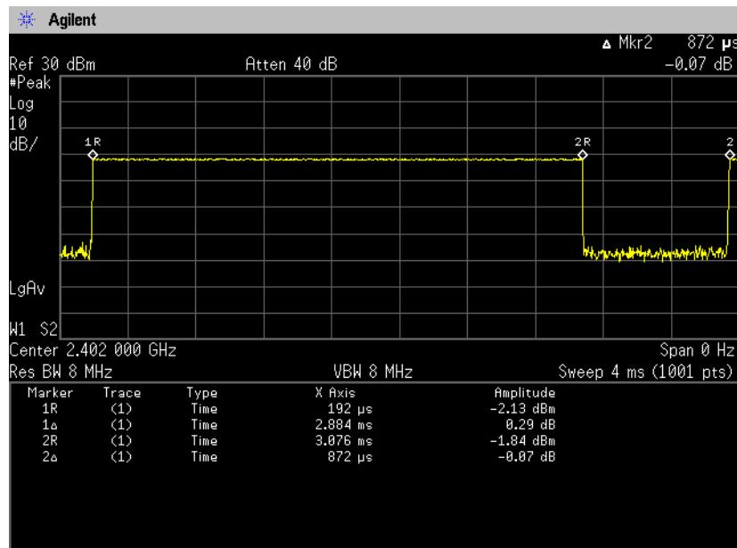
$$\text{Duty Cycle} = T_{\text{on}} / (T_{\text{on}} + T_{\text{off}}) = 2884[\text{us}] / (2884[\text{us}] + 872[\text{us}]) = 76.8[\%]$$
