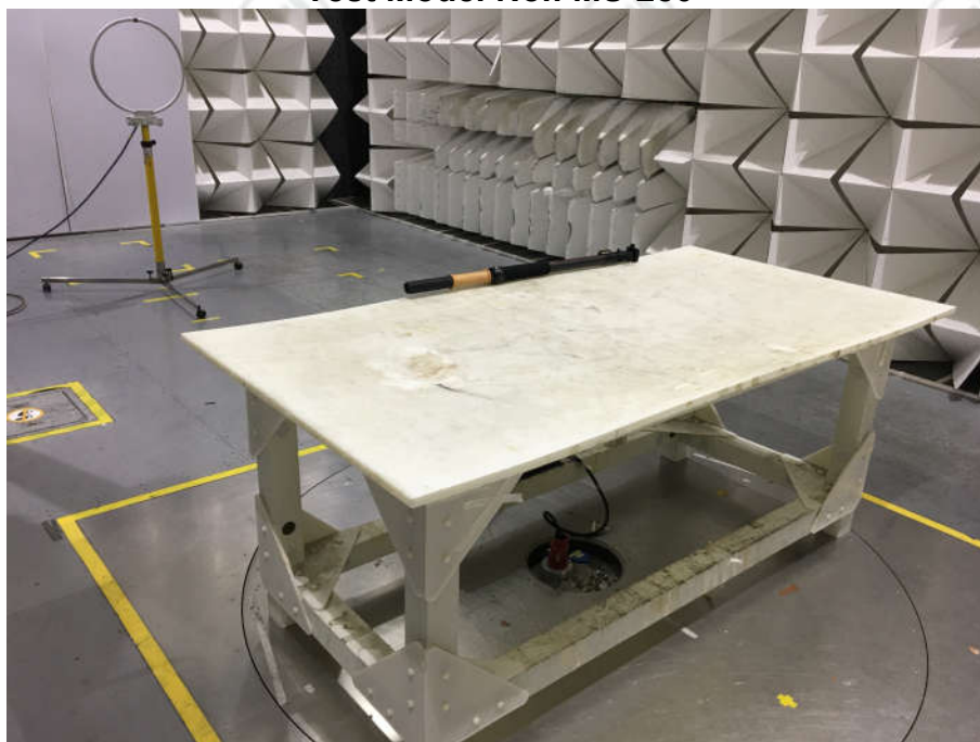
Radiated spurious emission Test Setup-1(Below 30MHz)
