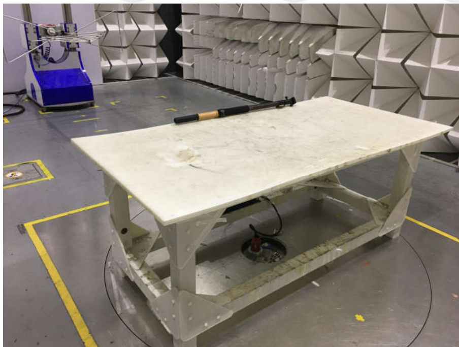
Radiated spurious emission Test Setup-2(Below 1GHz)
