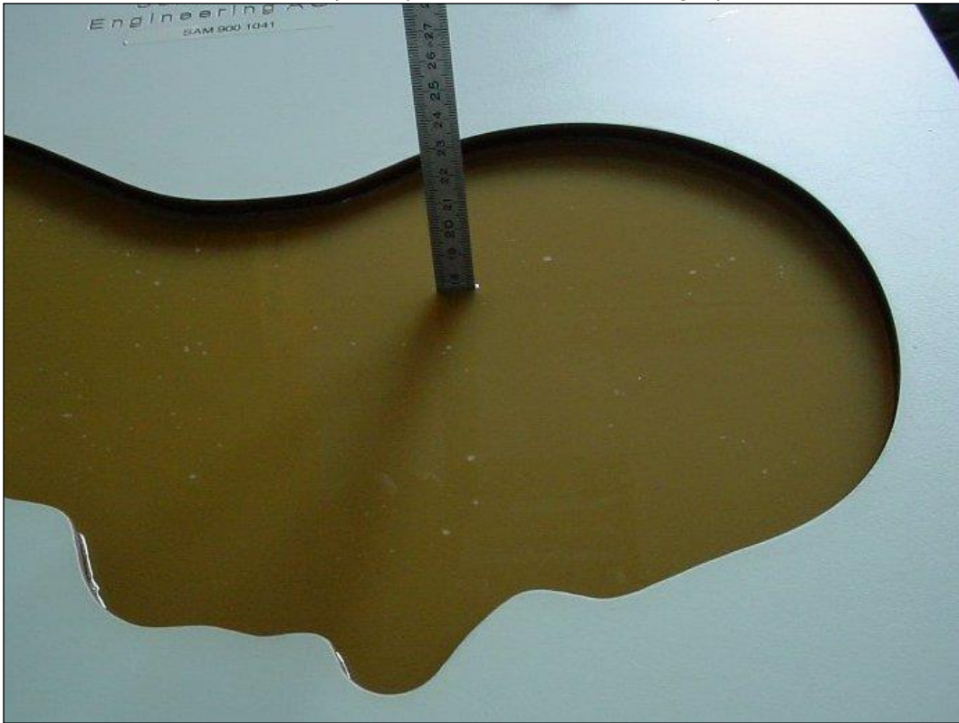
Photo 4: Liquid depth 5 GHz body simulating liquid
