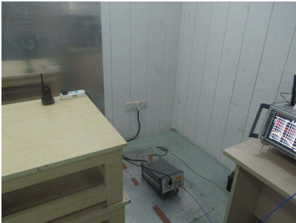
CONDUCTED EMISSION TEST SETUP
