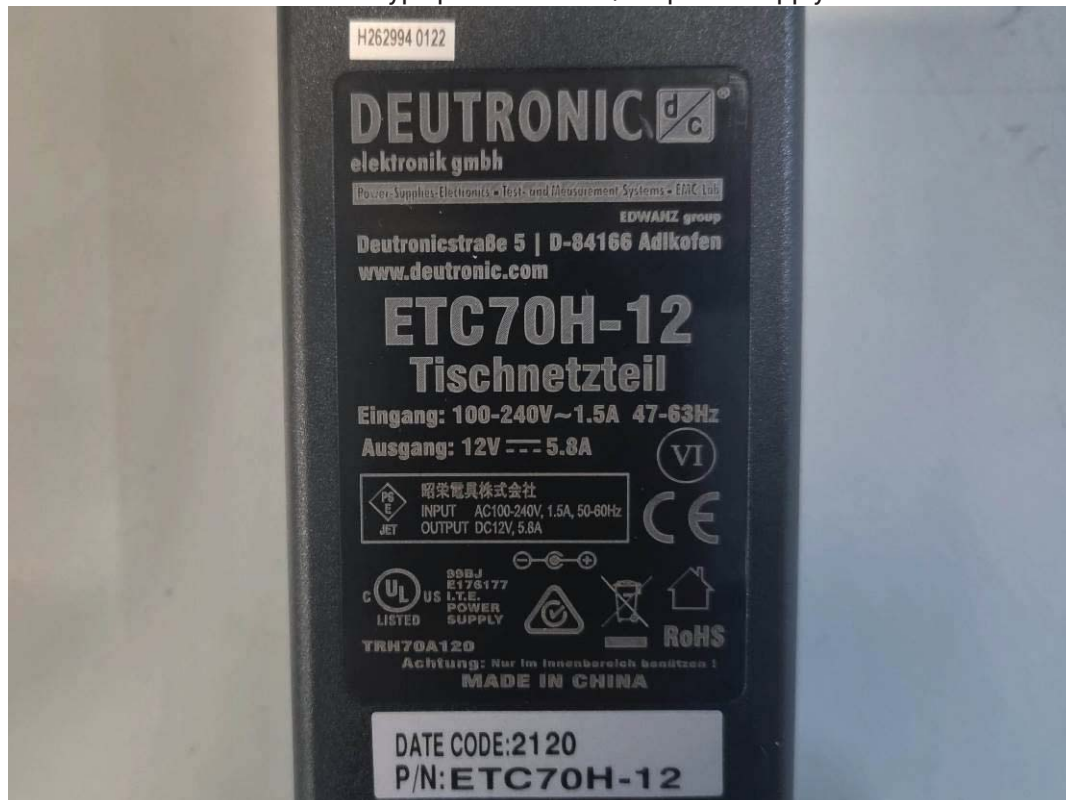
Photo 13: type plate of the AC/DC-power supply
