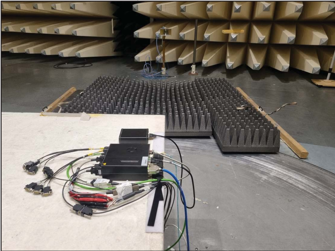
Photo 3: setup of radiated emission >1 GHz
