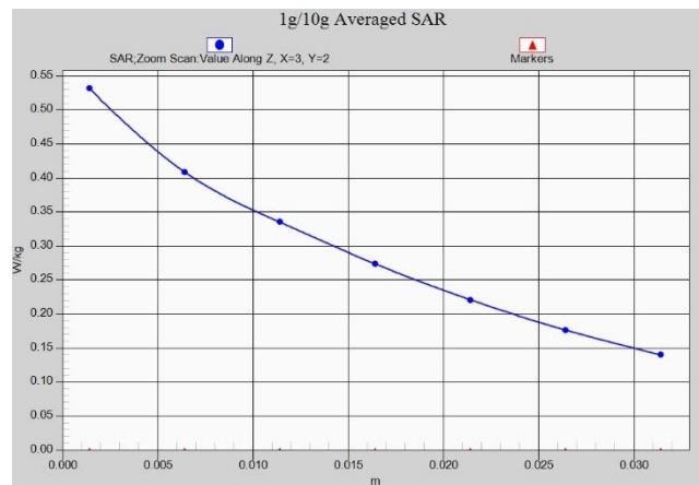
Fig. A-13 Z-Scan at power reference point (LTE Band 12)
