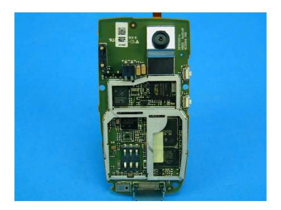
Sagem MC2004a - Rear PCB View 1 (Can Removed)
