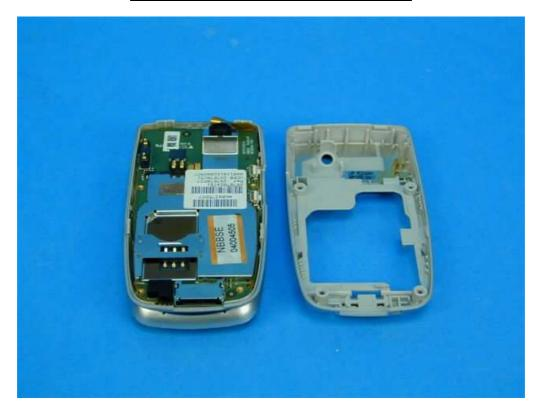
Sagem MC2004a - Rear PCB View 1 (Cover Removed)
