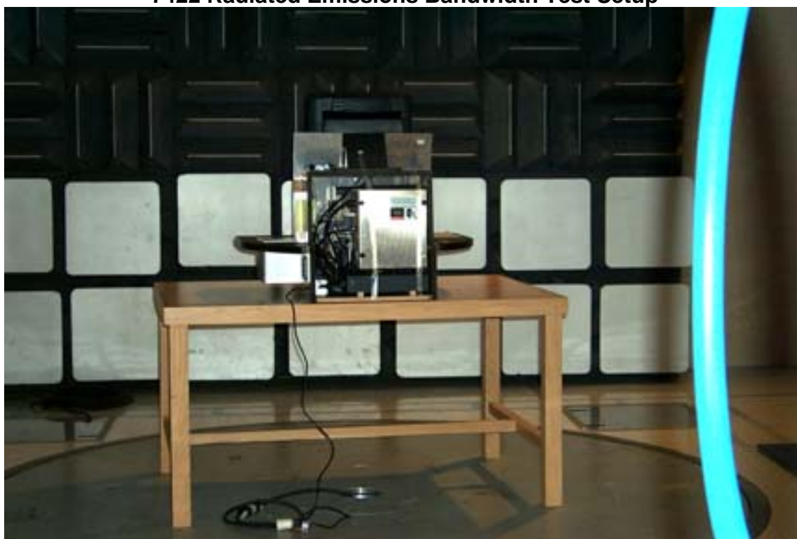
7422 Radiated Emissions Bandwidth Test Setup
