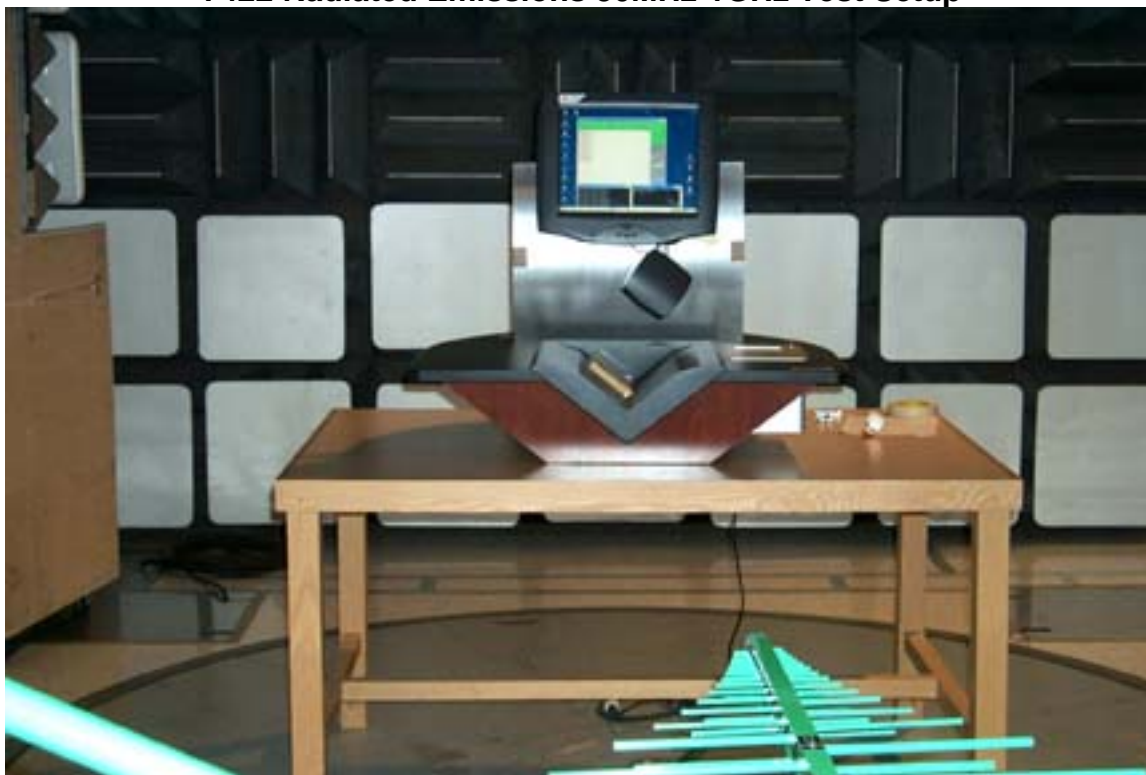
7422 Radiated Emissions 30MHz-1GHz Test Setup
