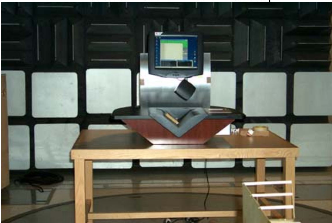
7422 Radiated Emissions 1GHz-5GHz Test Setup
