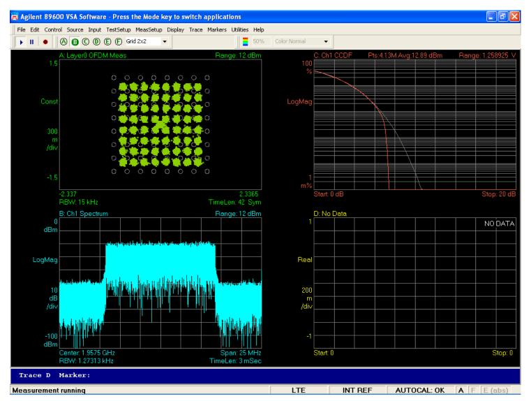
LTE QPSK Tx1 1982.5 MHz, 60W (47.8 dBm), 15 MHz BW
