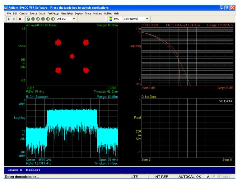
LTE 16QAM Tx1 1957.5 MHz, 60W (47.8 dBm), 15 MHz BW
