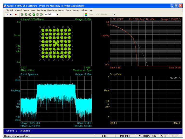
LTE QPSK Tx1 1957.5 MHz, 60W (47.8 dBm), 15 MHz BW
