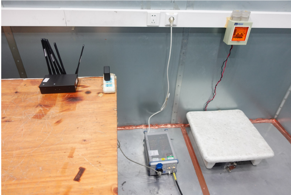
Picture 2 Conducted Emission Test Setup
