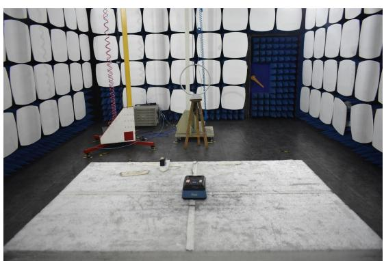
3. Radiated emission (9KHz-30MHz)
