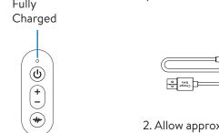
2. Allow approximately 3.5 hours to fully charge the battery (red light indicator will turn off).
