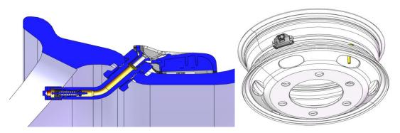
The sensor periodically reads pressure and temperature information. And the sensor periodically sends data via 433.92MHz RF signal.
