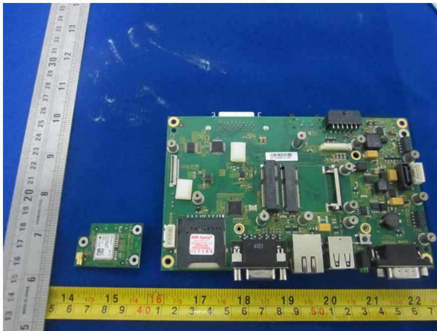
EUT –GPS Chip Uncover View
