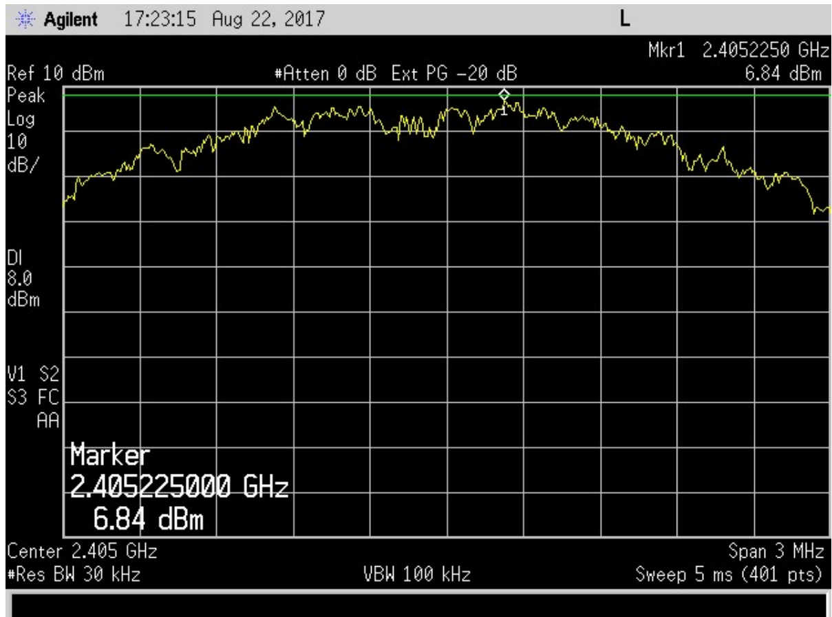
Figure 23. Peak Power Spectral Density - Part 15.247 (e) - Low Channel
