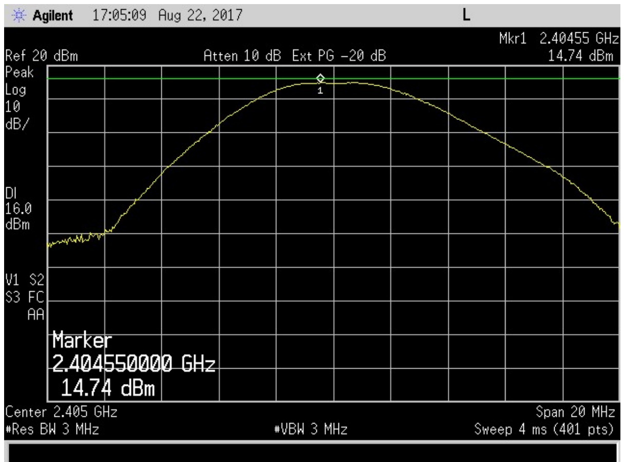
Figure 20. Peak Antenna Conducted Output Power, Low Channel
