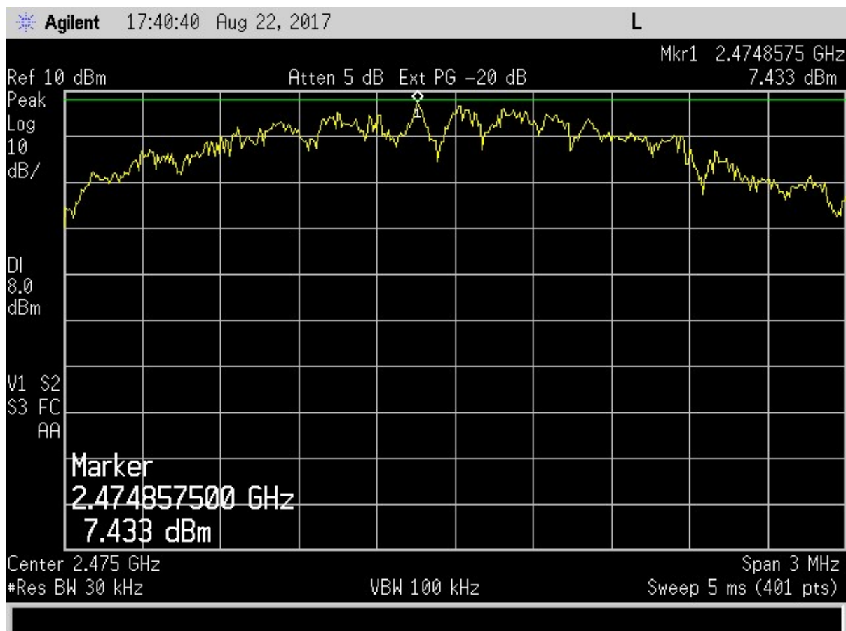
Figure 25. Peak Power Spectral Density - Part 15.247 (e) - High Channel
