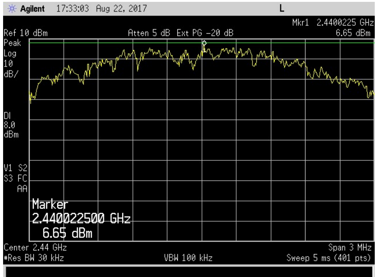
Figure 24. Power Spectral Density - Part 15.247 (e) - Mid Channel
