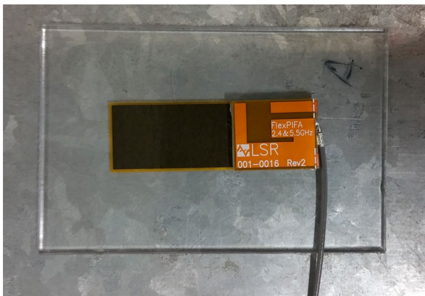
Figure 37: FlexPIFA mounted on metal Surface with 1.5 mm thick polycarbonate spacer
