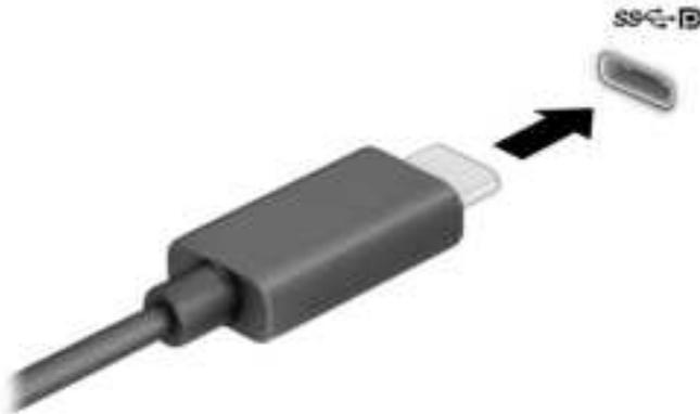
2. Connect the other end of the cable to the external DisplayPort device.
