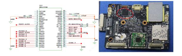
2. Changed the single-chip microcomputer chip(U16) from NUC029LAN to HHD32F103CBT5.
