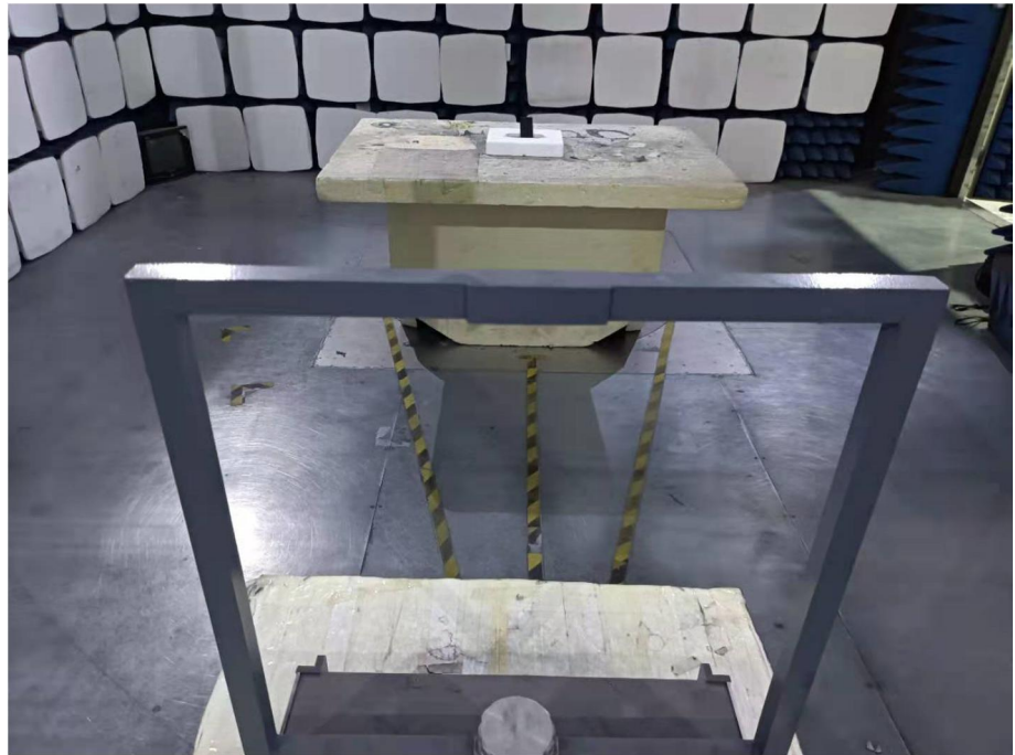
Radiation Emission Test Setup (Below 30MHz)
