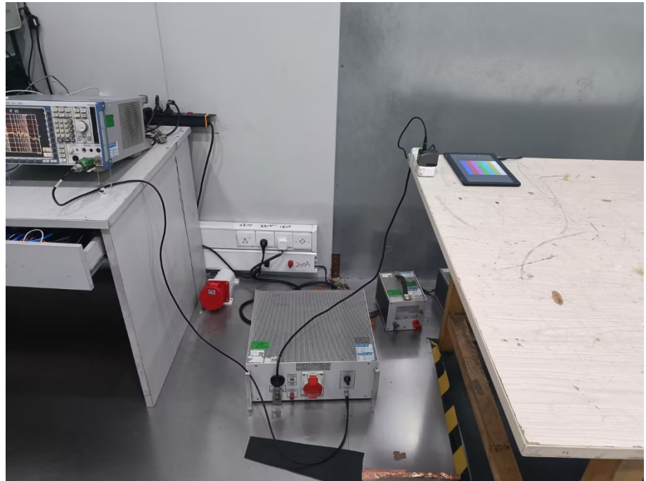
Conducted Emission Test Setup
