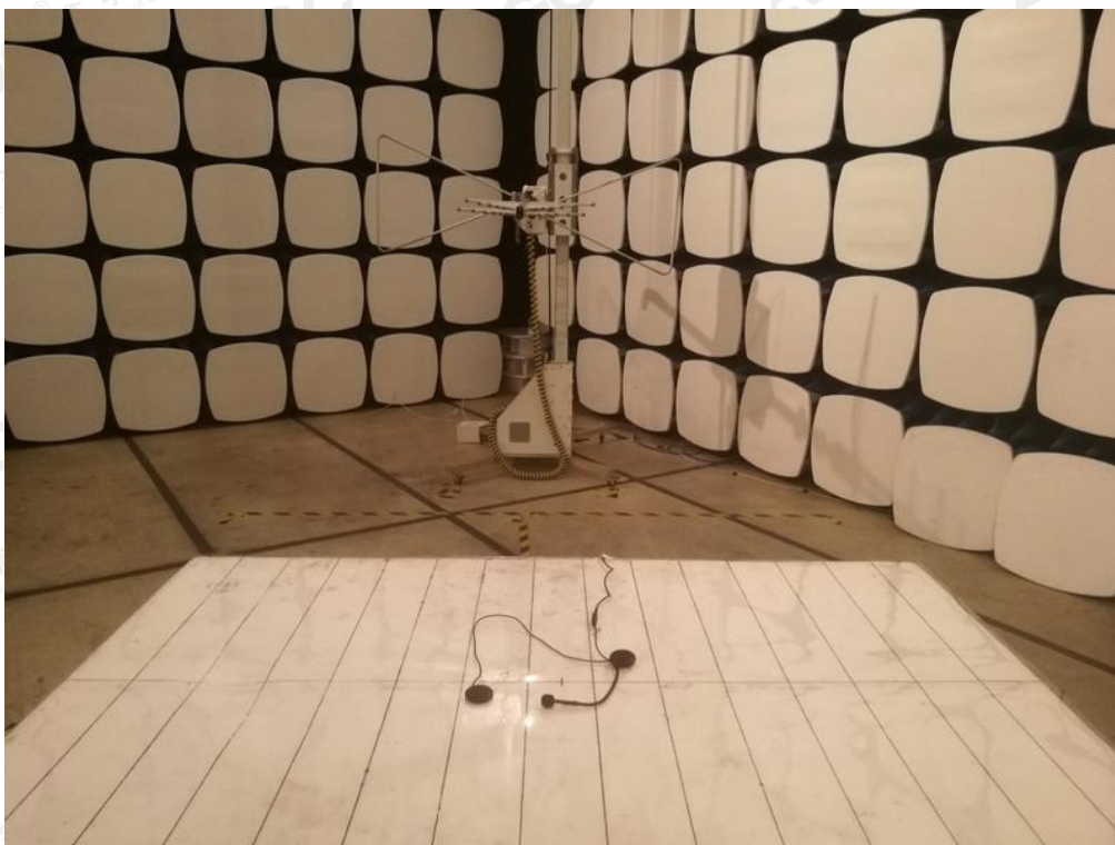
FCC RADIATED EMISSION TEST SETUP
