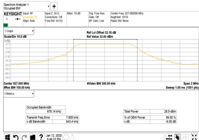
Plot 7.1.3 6 dB bandwidth test result at high frequency
